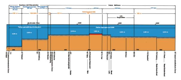
Figure 2: Longitudinal section of the Rhine (Source: WSV)
