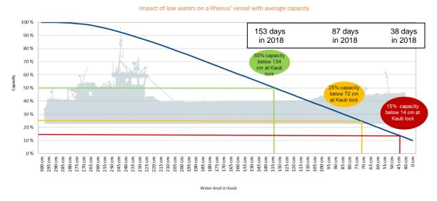
Figure 11: Fleet capacity vs water levels at Kaub (Source: Rhenus Logistics)
