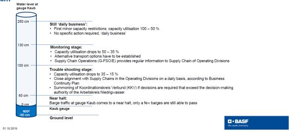
Figure 17: BASF decision-making chain in case of low waters (Source: BASF)
