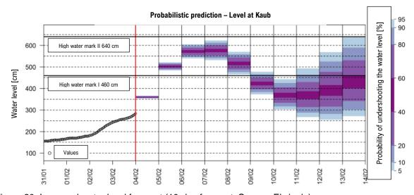
Figure 20: Improved water level forecast (10-day forecast, Source: Elwis.de)
