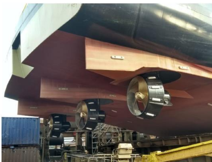
Figure 21: Aft ship design with 3 thrusters, reducing propeller diameter for low water operation (Source: MARIN, Photo: S. Oudakker, Oudcomb)
