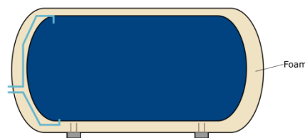
Figure 25: Pressure tank (foam insulated)
